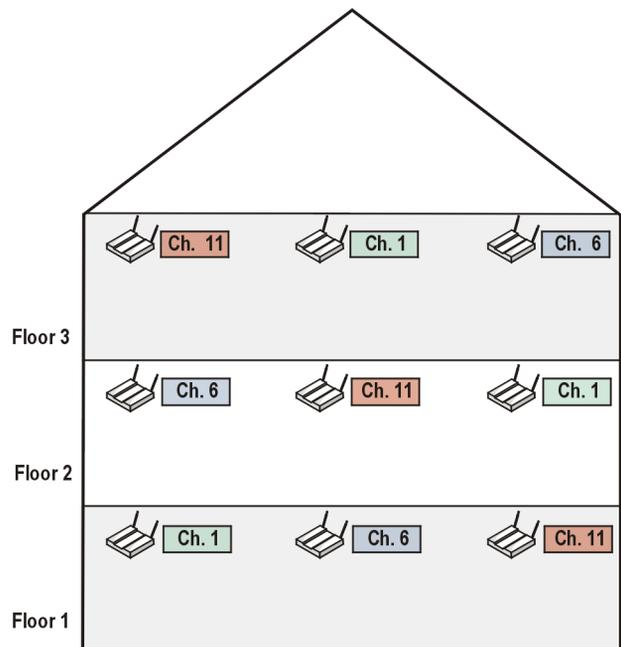
**Figure 5. Sample Frequency Topology Using Channels 1, 6, and 11**
