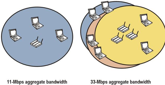
**Figure 3. Scaling Aggregate Bandwidth from 11 to 33 Mbps in a Localized Area by Colocating Three APs**
